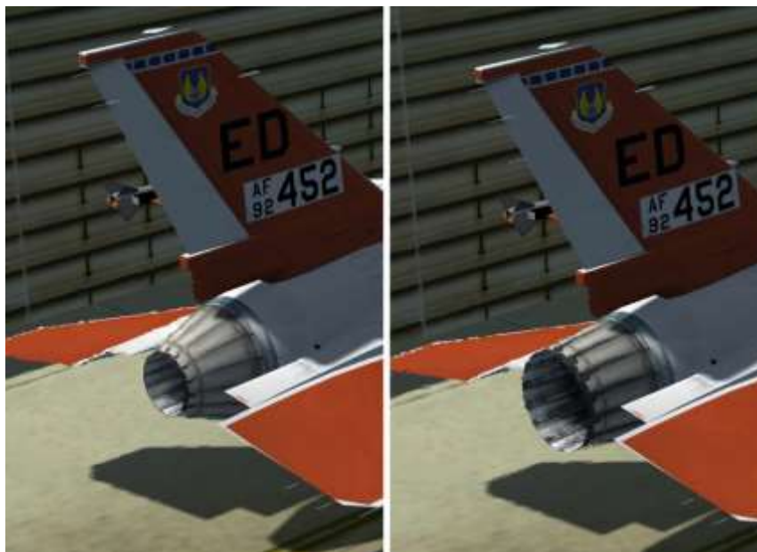
Performing the SEC check, nozzle closing & opening
