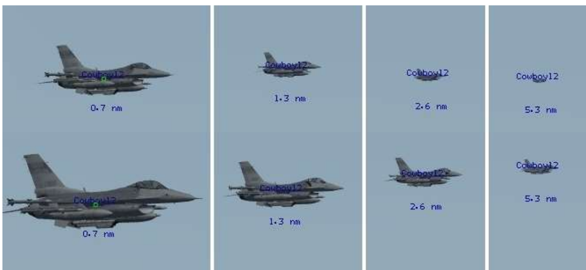
The above picture illustrates smart scaling off (top) and on (bottom) at several different visual ranges.
