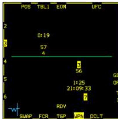
Assigned new location to HARM on station 7 from UFC while 1st HARM is in flight
