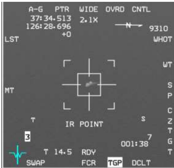
Figure 100 POINT track - TGP attempts handoff (HANDOFF IN PROGRESS shown on WPN page)
